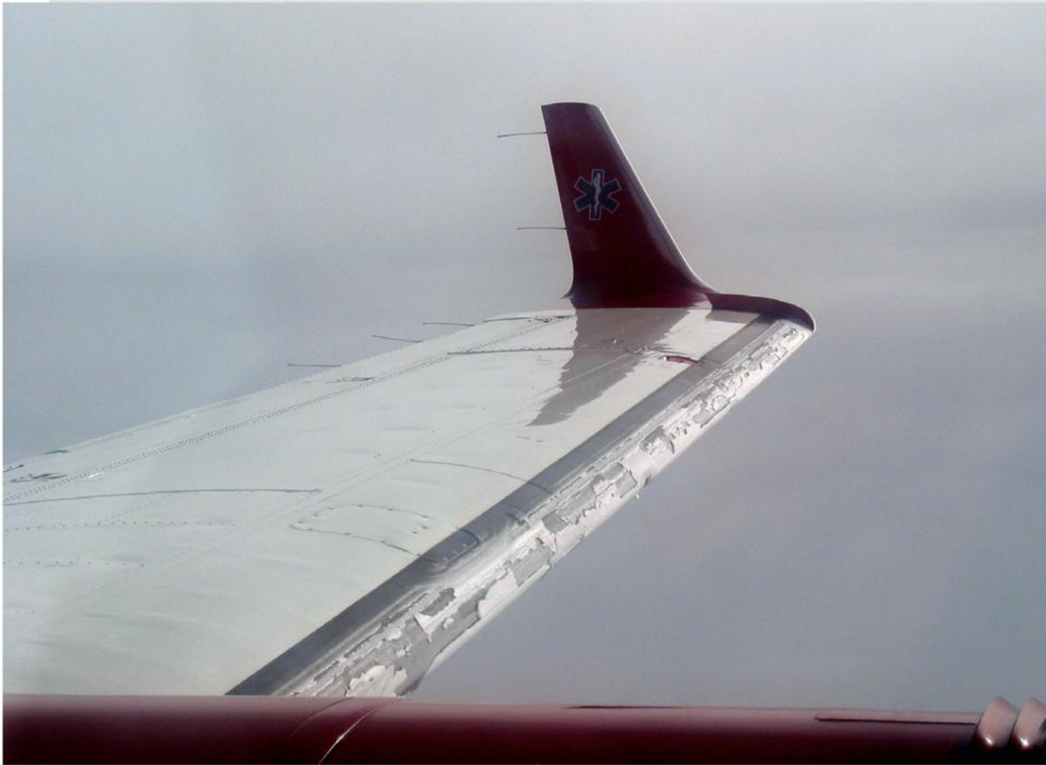
Klareis an den Tragflügeln einer Beechcraft King Air, © By Shawn from Airdrie, Canada - Some Ice on the boots, CC BY-SA 2.0, https://commons.wikimedia.org/w/index.php?curid=31604840
