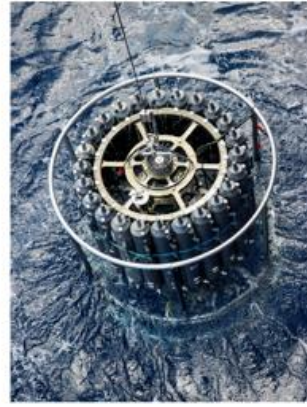
◀ Photo 3.13-3: A water sampling rosette with 24 closed water samplers returns to the surface from a water depth of over 4,000 metres.
