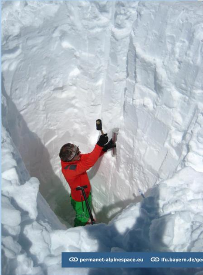
◀ Photo 4.6-2: Sampling of snow for determination of snow cover density in spring
