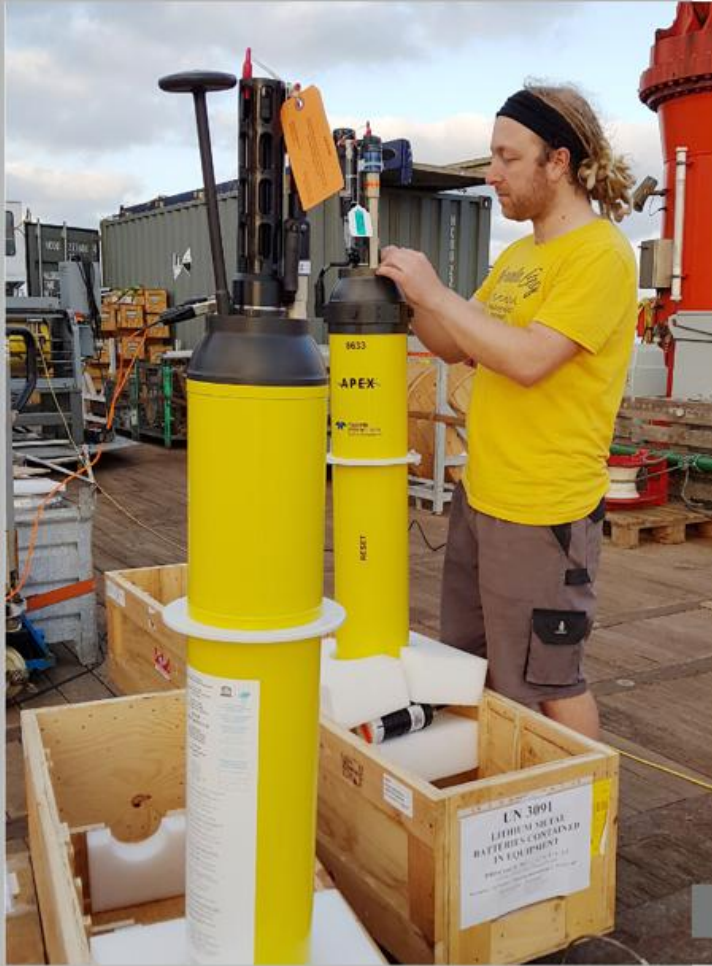
◀ Photo 3.13-2: Dr Bjorn Fiedler from GEOMAR prepares Argo deep floats with various biogeochemical sensors for deployment in the tropical Atlantic.
