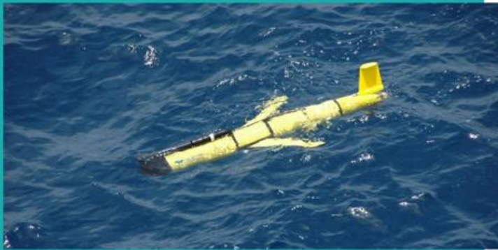
◀ Photo 3.2-1: A glider sending measurements from its successful dive for transmission via satellite. During its months-long missions, a glider measures vertical profiles of a multitude of ECVs at hourly intervals down to a depth of 1,000 m.
