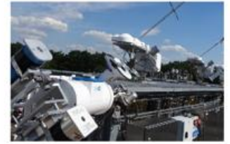
▲ Photo 2.5-2: Precision measurement devices for incoming radiation at Lindenberg BSRN station
