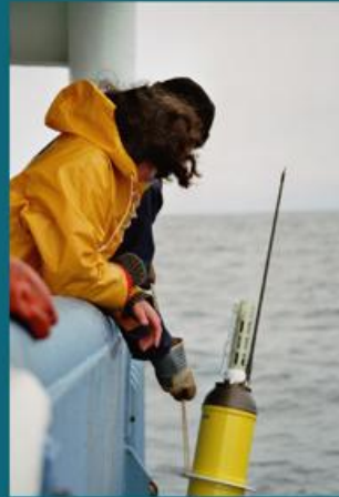
◀ Photo 3.2-2: Launch of an Argo deep float into the sea. Once deployed for 3 to 5 years depending on the design, the float will collect vertical profiles of temperature and salinity from the surface down to a depth of 2,000 m as well as information about current flow at around 1,000 m down in the ocean every 10 days and transmit these to the global data centre for Argo. At present, the Argo observing network is being extended to measure biogeochemical variables and include applications for profiles down to a depth of 6,000 m.
