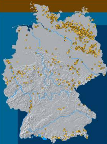
◀ Figure 4.4-2: Overview map of Germany with all 947 measuring sites in lake water bodies with a water surface of more than 50 ha and therefore subject to WFD reporting obligation. The samples are usually taken at the deepest point of the lake. (Source: BfG)
