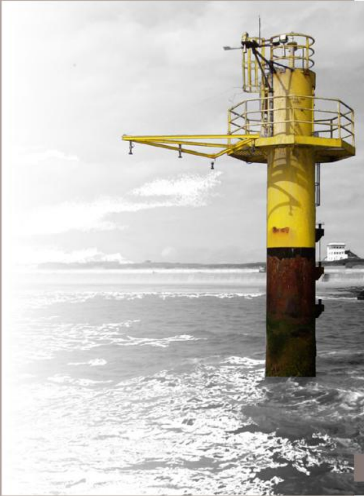
◀ Photo 4.1-3: Radar-based level gauge at Borkum/Südstrand with four measurement sensors
