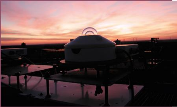
▲ Photo 2.5-1: Pyranometer for measuring global radiation at MOL-RAO
