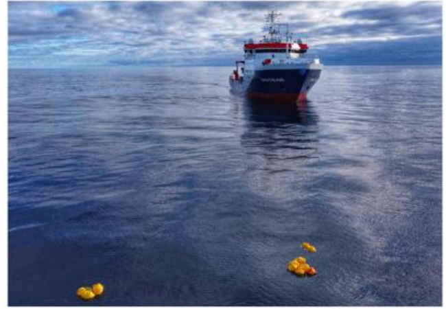
▲ Photo 3.1-2: The German research ship MARIA S. MERIAN approaching parts of a long-term mooring in the Labrador Sea. The sensors are raised once a year for maintenance. In addition, a wide range of ECVs are measured on board of the ship.
