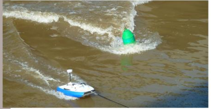
Photo 4.1-2: Runoff measurement by means of an acoustic Doppler current profiler (ADCP, in the foreground) during the Elbe flooding in 2013 ▶
