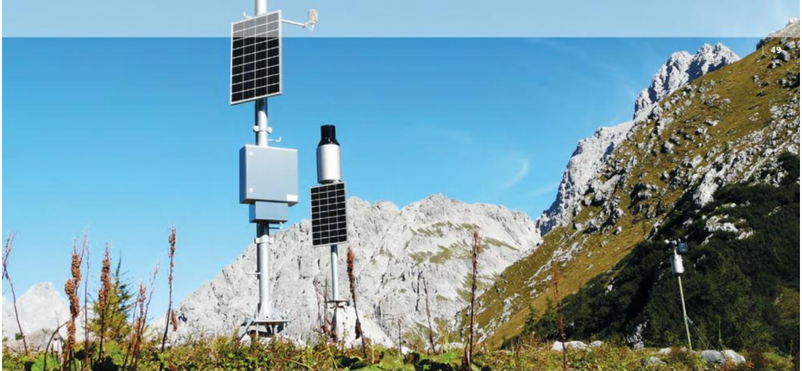
top Berchtesgaden National Park station Trischübel at 1,762 m; one of the DWD's mechanical wind measurement devices can be seen on the right.
