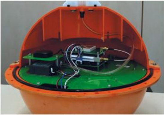
left Inside view of a drift buoy like the ones deployed by the frigate BAYERN
