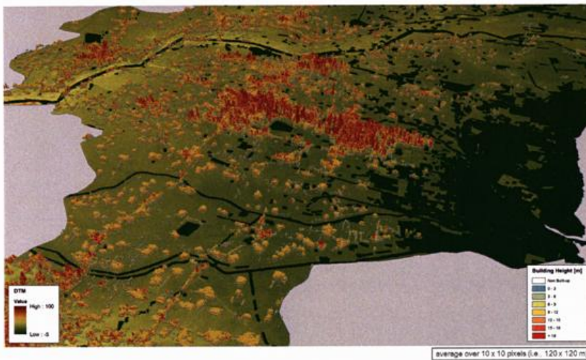
Fig. 3: Regional characterization of building volumes generated on the basis of TanDEM-X height data.
