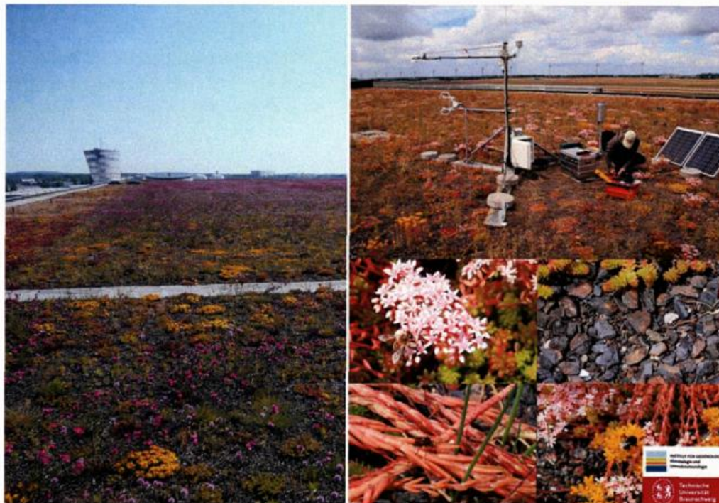
Fig.1: Impressions of the extensive green roof and the eddy covariance measurement station at the Berlin Brandenburg airport.
