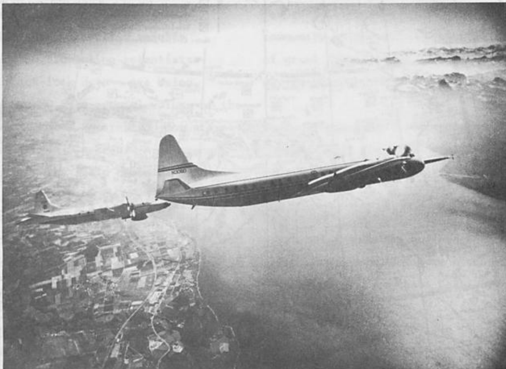
Fig. 4 Electra (right) and P-3 (left) turboprop aircraft (USA) as seen from Falcon jet aircraft (FRG) over Lake Geneva during intercomparison flight
