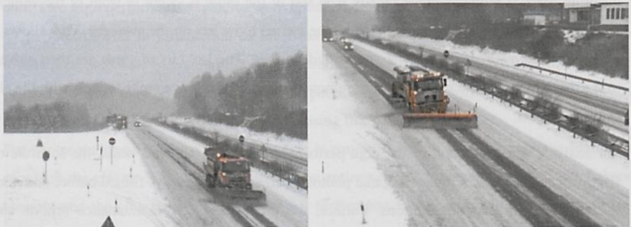
Figure 3: Clearance comparison of standard winter maintenance vehicle (left) and vehicle with high performance sweeper/air blast unit (right)
