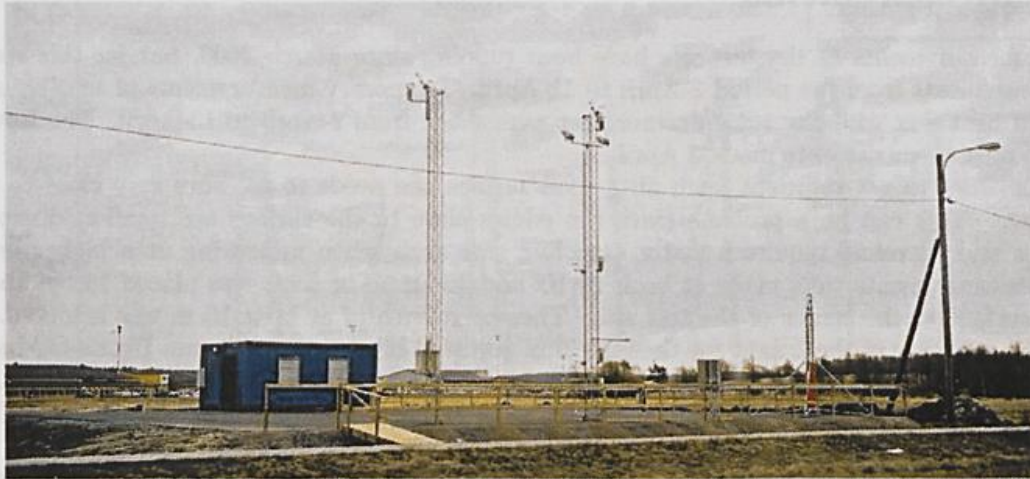
Figure 2: The asphalt surface at Säve as seen from the north-west. The RWIS-station is mounted on the left tower, while the instrument measuring the radiation components is on the right tower. The road is seen as a grey line in the foreground.
