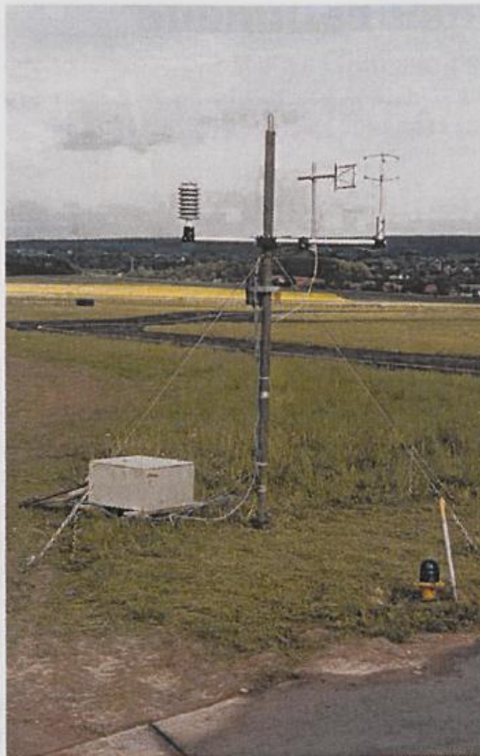
Figure 2: Measuring mast and box. The mast is equipped with a sonic anemometer/thermometer, a Krypton hygrometer, and a sensor for mean temperature/relative humidity (from right to left).
