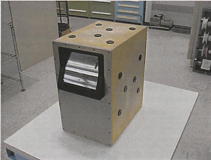
Figure 1: Picture of the new Laser Road Surface Sensor (LRSS)
