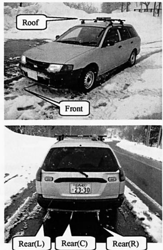
Fig. 2 The air temperature sensors attached to the vehicle in OBS-B.
