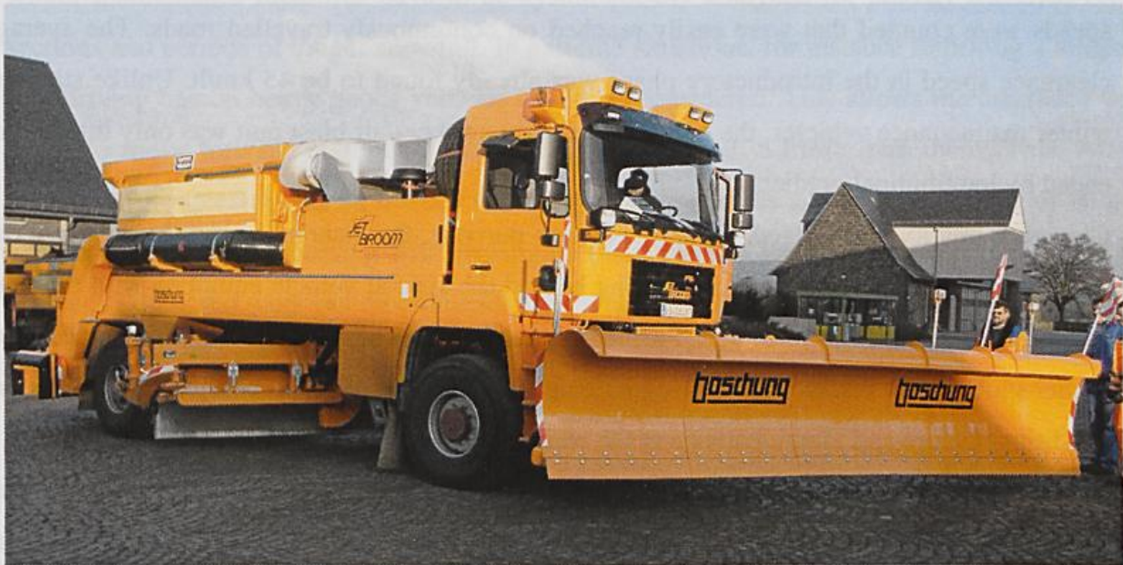
Figure 2: High performance sweeper/air blast unit being used in a winter maintenance vehicle
