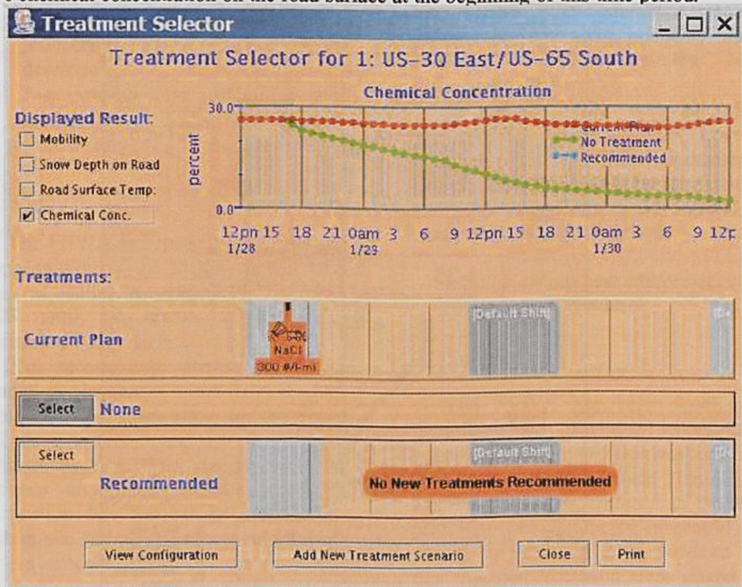
Figure 5 MDSS treatment selector screen. The red trace (top window) shows the predicted chemical concentration if the treatment application is followed. The green trace shows the chemical dilution rate if no chemicals were applied. Note that a prior application has left a 28% chemical concentration on the road surface at the beginning of this time period.
